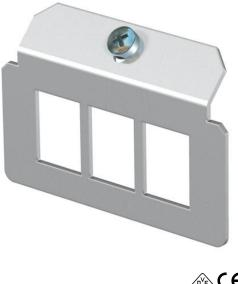
Support plate to accept three data connection modules of the following types: AMP TYCO: SL series 110Connect and Toolless, AMP-Twist; Brand-Rex: unshielded; GG45; TKM RJ MOD; Nexans: LANmark with Adapter Clip. Dimensions of a mounting opening in mm: 20.10 x 14.80.
