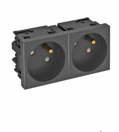
Socket with earthing pin and side connection, Double 33°, with increased touch protection, with screwless terminals, 2-pin, 16 A, 250 V~, with connection terminals to IEC 60884-1.
