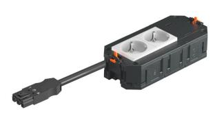
The ready-for-connection UTC3 universal support has 2 pre-installed 33° protective contact sockets in white of 16 A and one blanking cover for retroinstallation of an installation device of the Modul 45 or Modul 45connect series. Suitable for VL connection cables and device installation units of nominal size 2, 4, R4, 6 and D7
