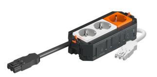
The ready-for-connection UTC3 universal support possesses 2 pre-installed  $33^{\circ}$  protective contact sockets in white of 16 A and one pre-installed  $33^{\circ}$  protective contact socket in orange of 16 A. Suitable for VL connection cables and device installation units of nominal size 2, 4, R4, 6 and R7.
